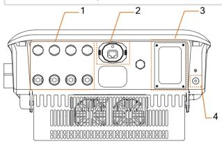
Fig. 3-1 Cable connection area
