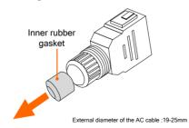
Step 4 Thread the AC cable of appropriate length through the waterproof terminal.
