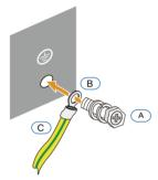
Fig. 3-3 Second PE connection
