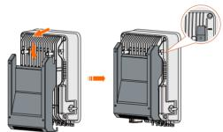
**Step 6 (Optional)** If you purchased a GPRS data acquisition module, install it to the communication interface of the inverter.
