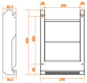
Fig. 2-1 Dimensions of the backplate (figures in mm)
