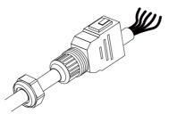
**Step 5** Connect the AC cable head to the European cold terminal by appropriate torque.
