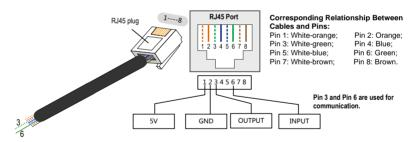
**Step 5** Verify the communication connection and configure the communication parameters.
