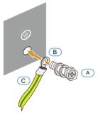
Fig. 3-3 Second PE connection
